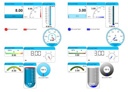
Fig. 4.2 Exemplary reactions of selected sidgets to the value of the upper (left) or lower (right) display limit being exceeded
