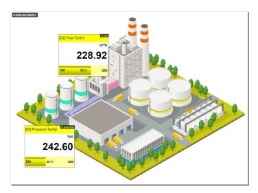
*Fig. 4.6 Visualization view during design* The HTML code responsible for the above effect is presented in listing 4.5.
