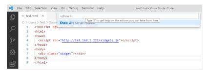
Fig. 3.6 Selecting the command to start previewing the current file
