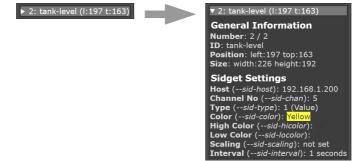
Fig. 4.4 Displaying additional information about the sidget
