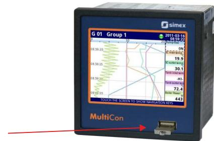
Enter **Menu** and **Device information** submenu, then move down the scroll bar and start the update process by pressing the **Firmware update** button.
