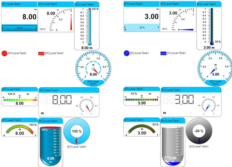
Fig. 4.2 Exemplary reactions of selected sidgets to the value of the upper (left) or lower (right) display limit being exceeded
